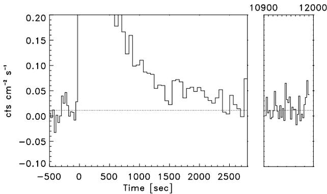
**Fig. 2.** 2–28 keV light curve of the long burst, zooming in at low flux levels and with a time resolution of 30 s. The dotted line indicates the out-of-burst persistent flux level. There are no data during times between the two panels.
