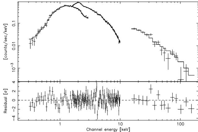
**Fig. 7.** *Top panel:* from left to right LECS, MECS and PDS spectrum (crosses with vertical lines depicting  $1\sigma$  error bars) and best fit result for power law and black body model (histogram). *Bottom panel:* fit residuals.
